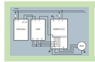
This version is simply controlled using the freely configurable I/O from a variety of sources such as a local operator station or from the MICROSYSTEMS LOGO module and the drives fixed frequency selection function. These units are all equipped with the following.
