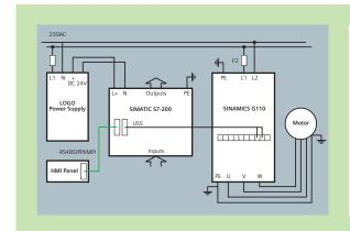
This version connects up to 31 drive nodes directly to the S7-200 via the integrated RS-485 port. Control instructions such as start/stop signals and the speed reference are simply transferred without the need for hardwiring of control cables. In addition other information such as status and parameter information can be simply passed between the nodes (eg to be displayed on an HMI panel)
