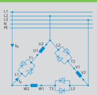
Rated current  $I_{\rm e}$  of the starter corresponds to 58 % of the rated motor current  $I_{\rm N}$
