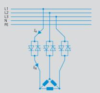
Rated current  $I_{\rm e}$  of the starter corresponds to the rated motor current  $I_{\rm N}$  3 cables to the motor
